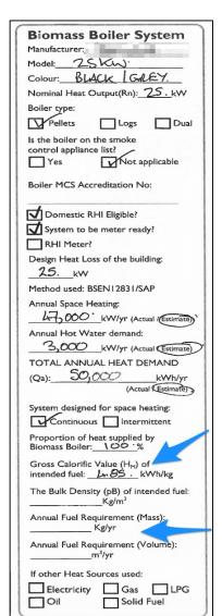
**Example 1:** this estimate does not include a predicted value for fuel mass or volume, no seasonal efficiency and the calorific value of fuel in kWh/kg is specified as 4.85kWh/kg. This was the only performance estimate given to customer before sale was agreed.
